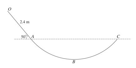
OABC is a vertical cross-section of a smooth surface. The straight part OA has length 2.4 m and makes an angle of  $50^{\circ}$  with the horizontal. A and C are at the same horizontal level and B is the lowest point of the cross-section (see diagram). A particle P of mass 0.8 kg is released from rest at O and moves on the surface. P remains in contact with the surface until it leaves the surface at C. Find
