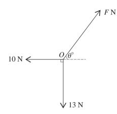
Three horizontal forces of magnitudes F N, 13 N and 10 N act at a fixed point O and are in equilibrium. The directions of the forces are as shown in the diagram. Find, in either order, the value of  $\theta$  and the value of F. [5]
